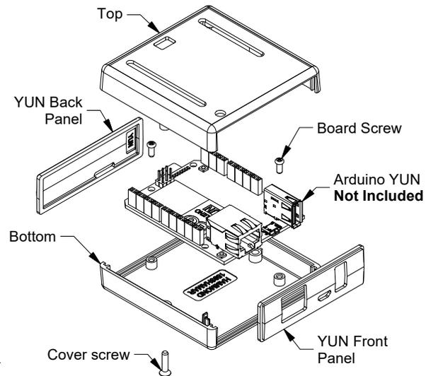
Enclosures can be Factory Modified (Milling, Drilling, Printing etc.) Contact Factory (modshop@hammondmfg.com) for quotes Solid models of this enclosure available in .stp or .x\_t (Part number and text placement/orientation on our products are subject to change, we do not recommend using them as a locating reference for modification purposes)
