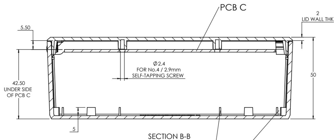
DOUBLE SUPPORT RIBS IN 4 CORNERS AND 2 OFF CENTRE, FOR PCBs A
